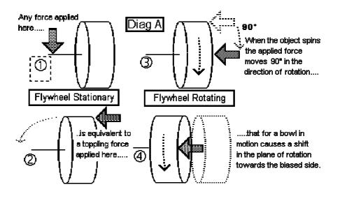
force at the top edge moves 90° in the direction of rotation, as shown in drawing 3. This causes the object to change its plane of rotation instead of toppling, as shown in drawing 4.
