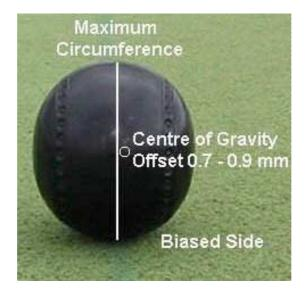
This offset provides an arm for a moment of toppling force created by the bowl's own weight. The moment of force is equivalent to a weight of about 23 grams tugging downward at the small disc. This moment of force constitutes the bias
