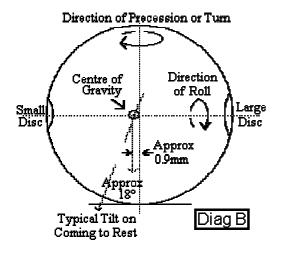
Diagram B shows how the same principle applies to biased lawn bowls. It shows the cross section of a bowl advancing towards the reader. The moment of the weight of the bowl acting downward from the offset centre of gravity creates a toppling force. This moment of force has a tendency to topple the bowl towards the reader's left. However
